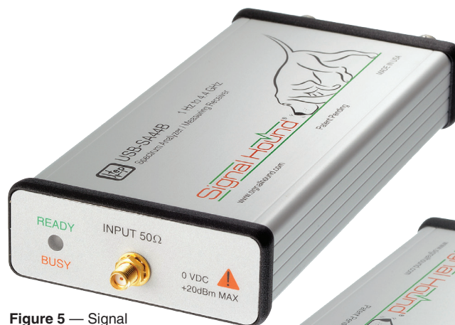
Figure 5 — Signal Hound USB-SA44B spectrum analyzer front panel. Note that the case graphics have changed since we bought the review unit, but the features and performance are the same.
