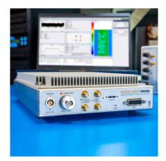
The SM435B is a high-performance spectrum analyzer and monitoring receiver. Tuning from 100 kHz to 43.5 GHz, the analyzer has 160 MHz of instantaneous bandwidth (IBW), 110 dB of dynamic range, 1THz/sec sweep speed at 30kHz RBW (using Nuttall windowing), and phase noise performance that is low enough to contribute less than 0.1% error to EVM measurements and rival even the most expensive spectrum analyzers on the market.
