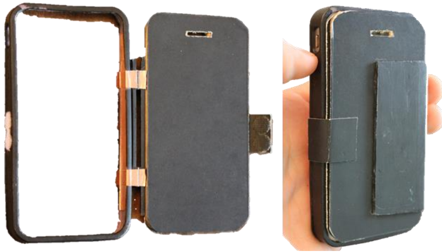
Figure 3. The self-constructed iPhone 4 Case with Plastic Hinge. This case secured with a Velcro fastener features an electromagnetic shielding flap that folds over the screen, redirects the signal along the hinge, grounds it to the phone's metal, and feeds it towards the back.
