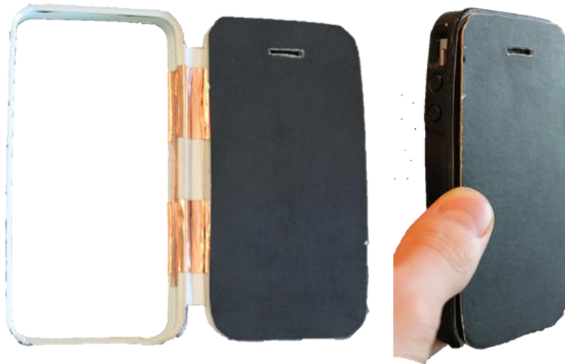
Figure 4. The self-constructed iPhone 4 Case with Paper Hinge. This case features the same shielding method as the other self-constructed case, but with a flexible flap that can be shifted to protect the back of the phone as well.
