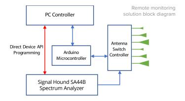
Our customer put together some C-code on an outdoor industrial computer to automate for periodic data collection. They integrated a small antenna rotator with an Arduino connected to the computer in order to select different antennas for re-evaluating the frequency spectrum. Thanks to the SA44B's size and power use, a battery-based micro-ATX Windows PC was able to control the entire solution.
