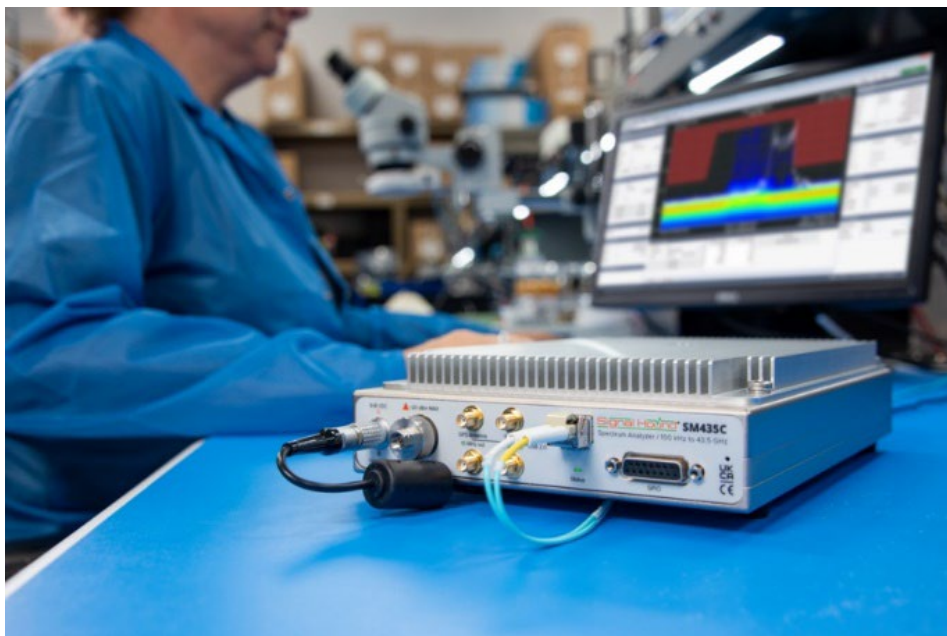
The SM435C with 10GbE is perfect for remote, network-connected analysis up to 43.5 GHz
