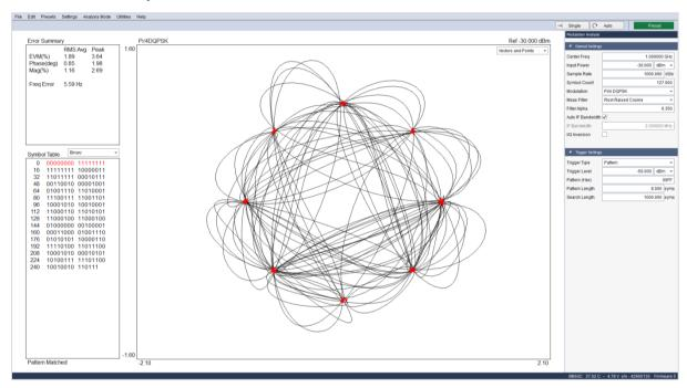
In 3.0.8 of Spike™ Spectrum Analysis software, constellation diagrams for signal analysis are now a standard feature that can aid in analysis of a wide range of digital modulations, including Pi/4 DQPSK.
