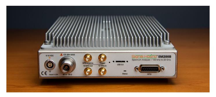
The SM200B is a high-performance spectrum analyzer and monitoring receiver. Tuning from 100 kHz to 20GHz, the analyzer has 160 MHz of instantaneous bandwidth (IBW), 110 dB of dynamic range, 1THz/sec sweep speed at 30kHz RBW (using Nuttall windowing), and phase noise performance that is low enough to contribute less than 0.1% error to EVM measurements and rival even the most expensive spectrum analyzers on the market.
