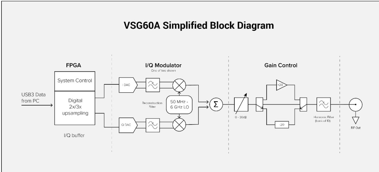
2 GHz (and a small segment around 800 MHz), driven by a dual channel DAC. The DAC clocks in I/Q samples at 66-102.4 MSPS. The data rate from the PC to the FPGA is 22-51.2 MSPS I/Q, so inside the FPGA we digitally up-sample by a factor of 2 or 3. This allows the use of a single optimized reconstruction filter for typically better than 60 dB rejection of any aliased baseband signals, and allows the PC to efficiently up-sample the user-selected baseband clock rate by a simple power of two.
