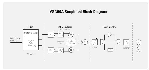
2 GHz (and a small segment around 800 MHz), driven by a dual channel DAC. The DAC clocks in I/Q samples at 66-102.4 MSPS. The data rate from the PC to the FPGA is 22-51.2 MSPS I/Q, so inside the FPGA we digitally up-sample by a factor of 2 or 3. This allows the use of a single optimized reconstruction filter for typically better than 60 dB rejection of any aliased baseband signals, and allows the PC to efficiently up-sample the user-selected baseband clock rate by a simple power of two.
