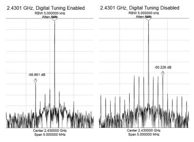
To mitigate these spurs, a low spur mode has been added, which is on by default. When low spur mode is enabled, the fractional-N PLL uses a very low denominator to keep the spurs at least 2 MHz away from the carrier and typically below -50 dBc above 3.7 GHz, and below -55 dBc below 3.7 GHz. This gives a coarse LO frequency, which is then digitally tuned to the exact requested frequency. The advantages of digital tuning are very low-level, predictable
