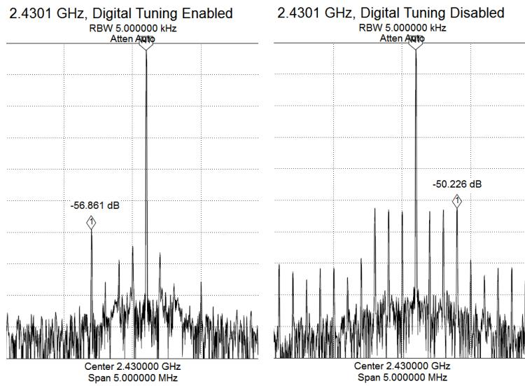
advantages of digital tuning are very low-level, predictable fractional-N and integer boundary spurs, and nearly infinite tuning resolution. The disadvantage is that the hardware's I/Q offset is no longer centered in the modulation envelope.
