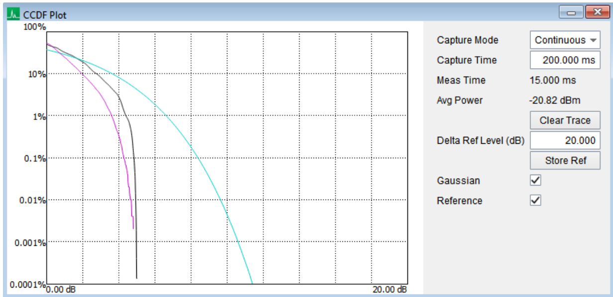
Figure 11: Comparing synthetic noise signal to a Gaussian reference and ideal test signal.
