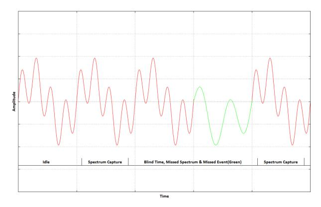
In this image we see an event missed due to the blind time between spectrum sampling. With Real-Time spectrum analysis we can prevent this and capture ALL possible events.
