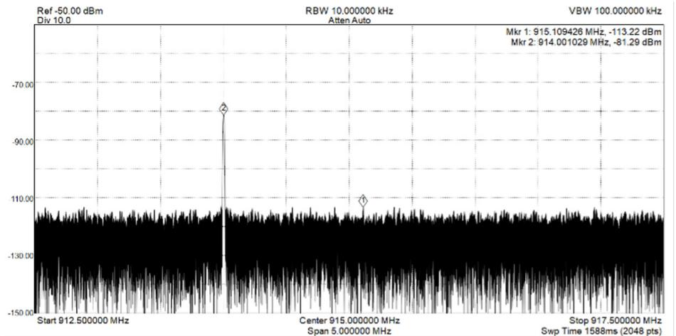
Figure 1a— $VBW > RBW$ ; RBW = 10 kHz, VBW = 100 kHz
