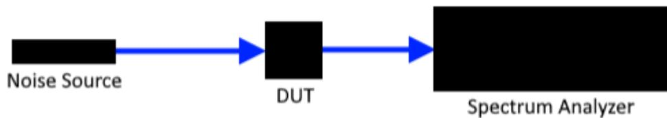
Figure 11: Diagram of DUT measurement step setup.
