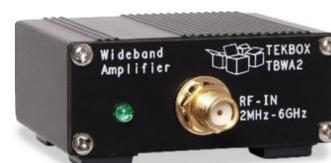
Figure 5: TekBox TBWA2 40 dB Wideband Amplifier.
