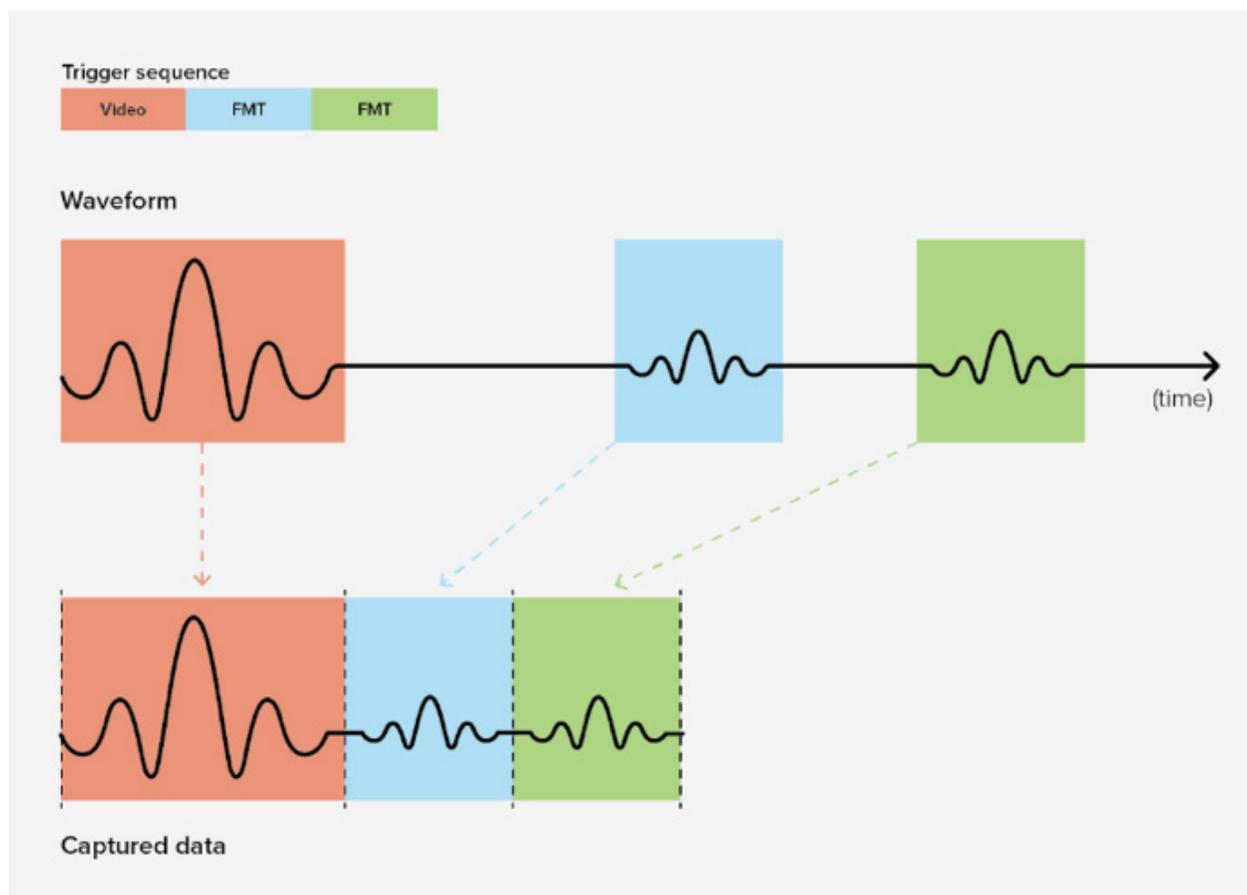
Figure 1 – The SM200B allows you to set up a variety of triggering combinations.
