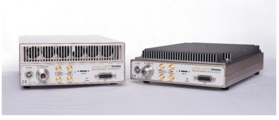
Signal Hound's SM200A 20 GHz spectrum analyzer now supports VITA 49 functionality
