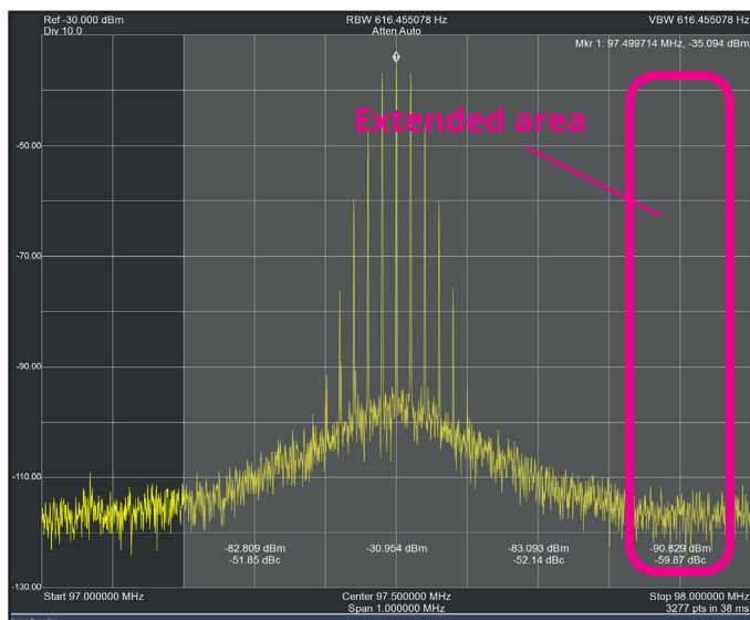
Figure 13—Changing the “Count” field in Spike to 4 or more extends the adjacent channel power ratio measurement beyond the immediately adjacent channels.
