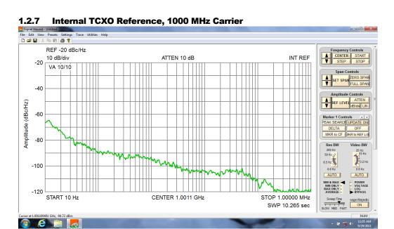
(Note: Plot starts at 10 Hz due to unstable readings below 10 Hz)
